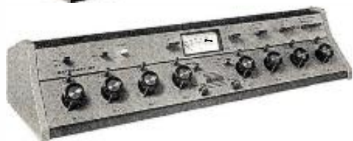
Gatesway 80 audio console: 18 inputs into 8 monaural mixing channels; modular solid-state amplifiers, step-type attenuators.
